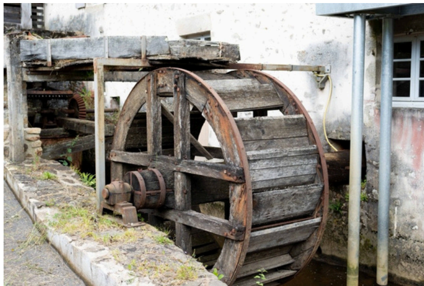
THE WATER WHEEL of GOT MILL: to be replaced soon by a modern metal wheel.
