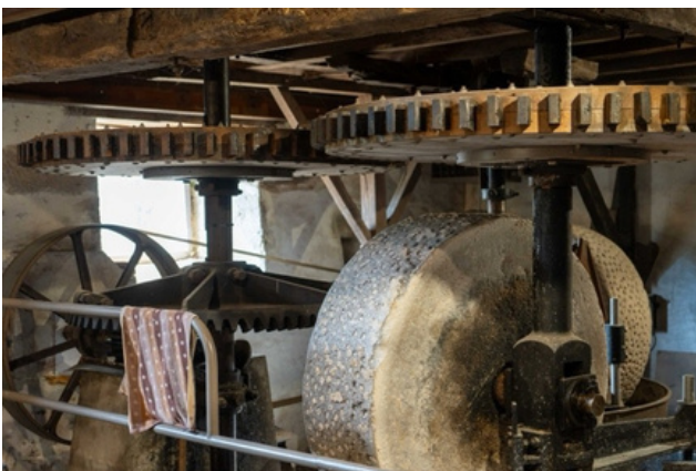
MACERATING THE WOOD TO PRODUCE THE PAPER USING ENERGY FROM THE WATERMILL
