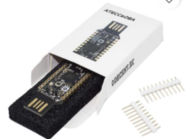
Pre-provisioned Secure Element (Microchip 608A)
